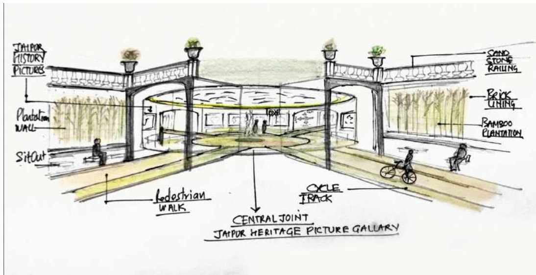
Figure 39: Sketch of Underpass for Pedestrian and Cycle Movement
